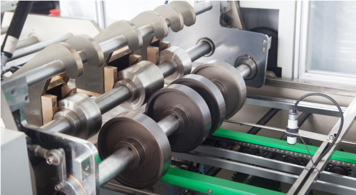
# The collecting frame can be opened in three parts. It is easier to install the forming spare part and commissioning.
