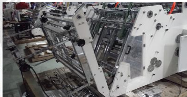
# The collecting frame can be opened in three parts. It is easier to install the forming spare part and commissioning.
